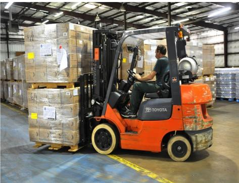
**Forklift Safety.** All forklift operators must be trained and certified. Equipment must be inspected, and all safe operating procedures must be followed. Drive slowly, and do not travel with elevated loads. Make sure all signal alarms work, and watch for hazardous conditions (involving both workers and objects). Be sure to wear your seatbelt.
